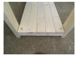
Centralise and secure using the screws supplied.
