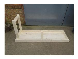
Lay the top upside down and place a leg in position as shown.
